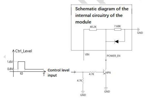
POWER\_EN foot and GND access module, MCU connected to the microcontroller, the motherboard power-up so that the control level output high, transistor conduction, POWER\_EN foot is low, the module does not start; power supply stabilization so that the control level has
