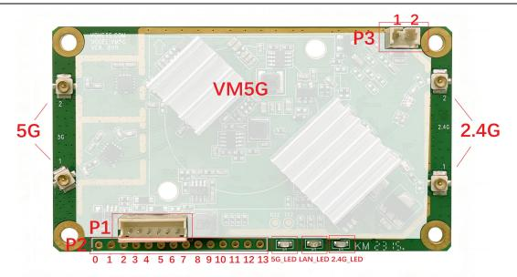
Note: Because the module is too small, the four metal screws are easy to lead to deformation of the module, chip desoldering, it is recommended to use plastic screws, and only used to locate can be, to leave a little room for manoeuvre!
