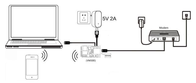
The Ethernet cable of **VM5G** module defaults to LAN port, you must set "WAN/LAN interchange" so that the Ethernet cable is WAN port to use the broadband dialing function.
