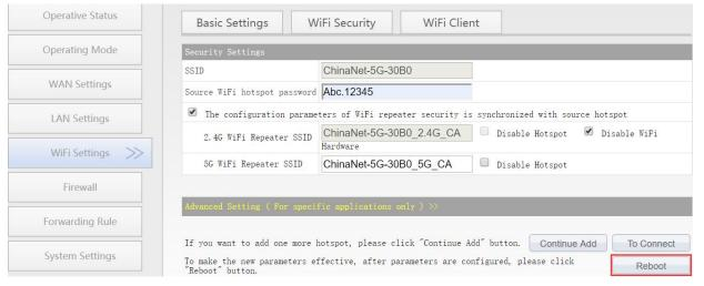
Remark 3: After VONETS module sets the WAN port to access the WiFi hotspot in the routing mode, its LAN port IP is still 192.168.254.254, and the terminal device also obtains the IP address of the same network segment, can login configuration page by 192.168.254.254 or http://vonets.cfg.
