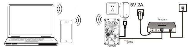
• VONETS module is used as a wireless router. WAN port can be set to connect to the WiFi hotspot for use as a secondary router.
