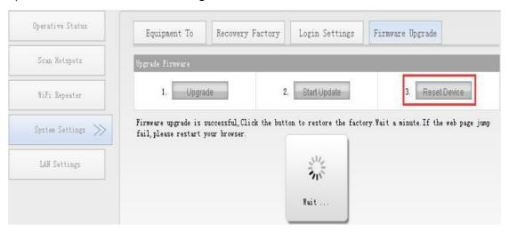
5. After restarting the device, wait for the VONETS device indicator to flash quickly, then reset the VONETS device again to complete the upgrade (press and hold the reset button for 5 seconds, then release, wait for the indicator to flash slowly -> stop -> finally resume fast flashing, the entire upgrade process is complete).
